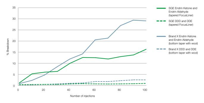
50 ppm Endrin and DDT test mix, 1 µL splitless injection at 250°C, HT grade septa (PN: 041898)
